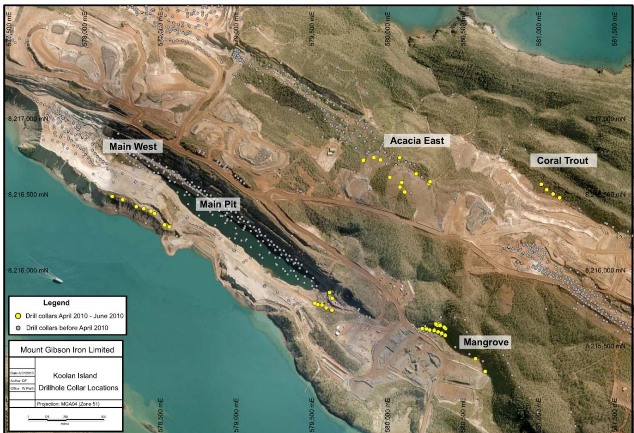
Figure 12 – Plan of Koolan Island showing drillhole collar locations for holes drilled during the quarter (yellow circles) and all previous drilling (grey)
