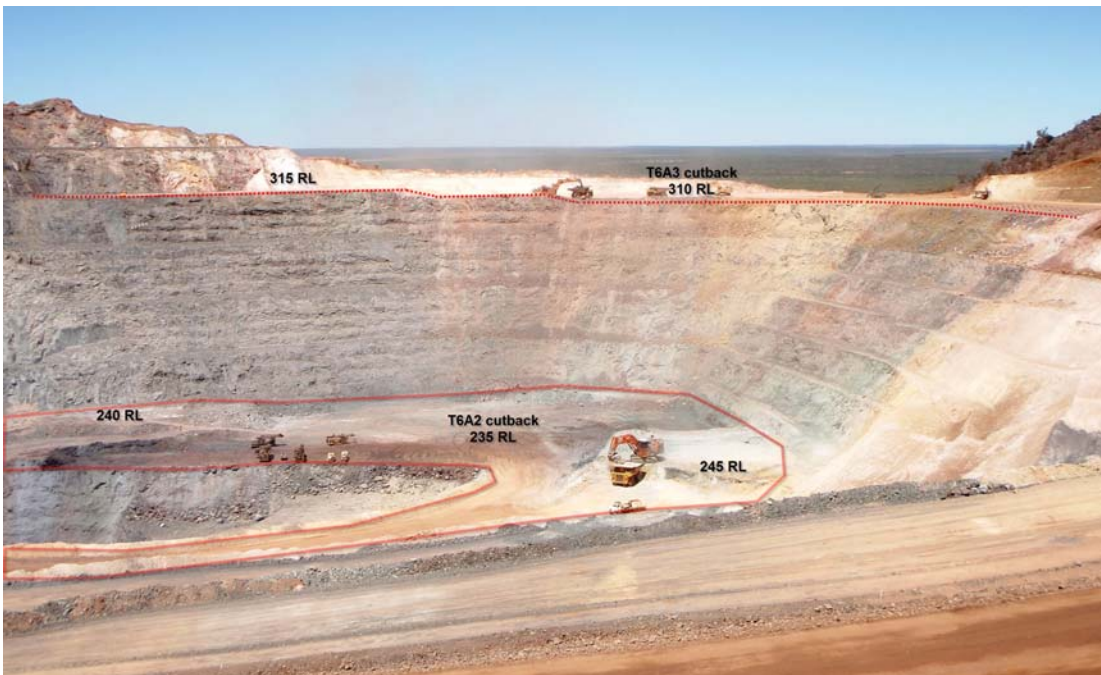
Figure 4 - T6A2 cutback from main range operation north wall
