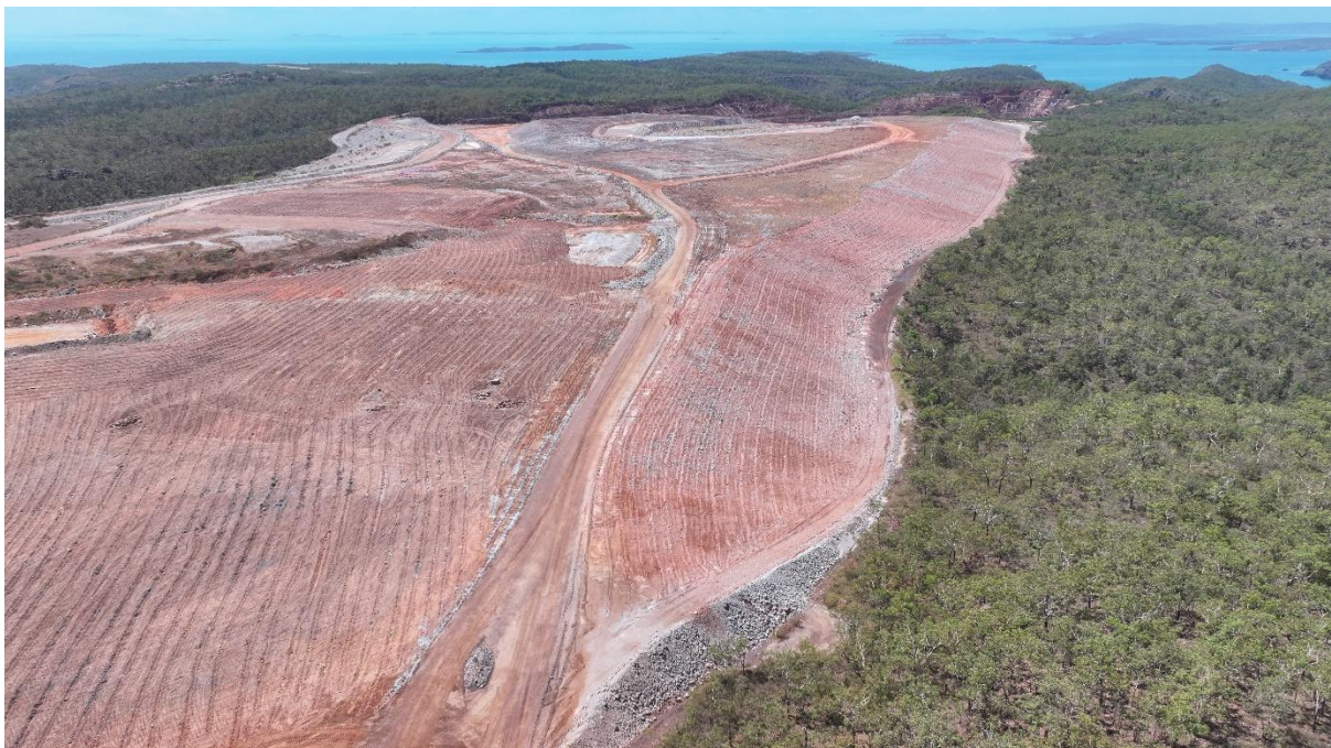
View looking northeast across the backfilled East and Barramundi Pits, and now-rehabilitated waste dump and stockpile areas, 15 October 2026
