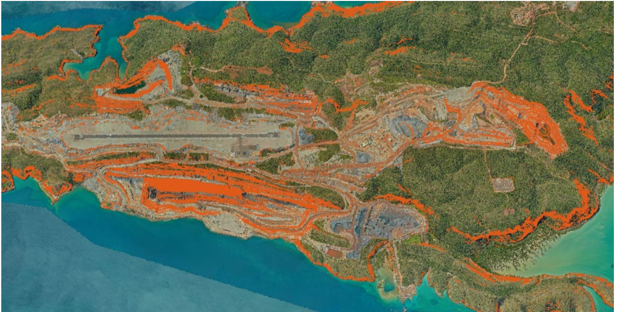
Figure 60: Slope assessment. Red highlighting indicates a slope of 37° or greater.
