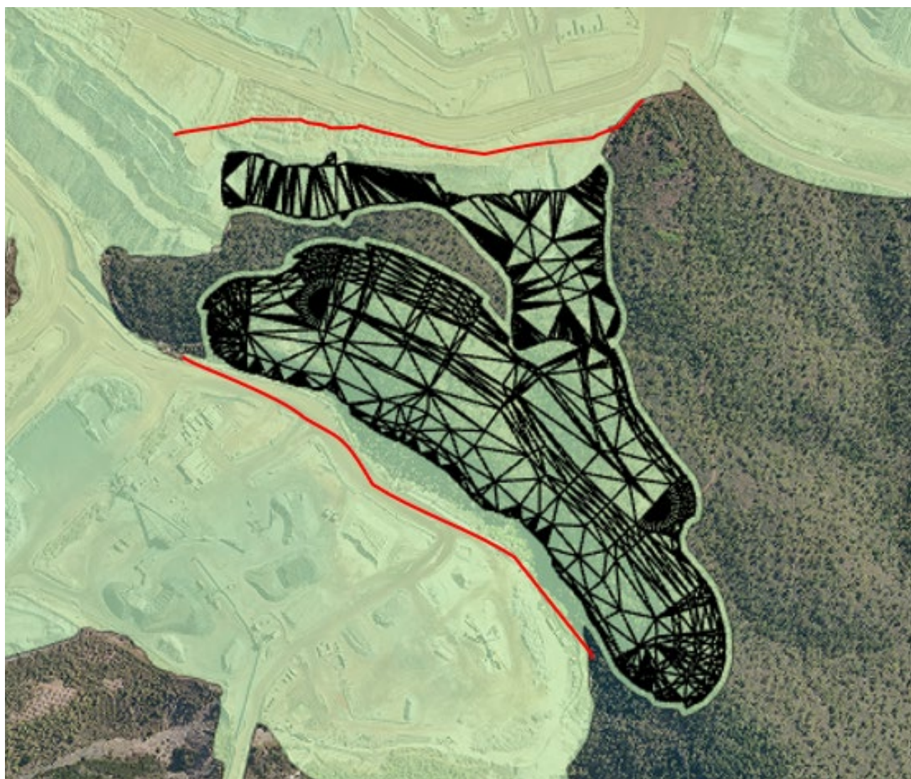
Figure 116: Conceptual location of the Mangrove deposit planned pit abandonment bund.
