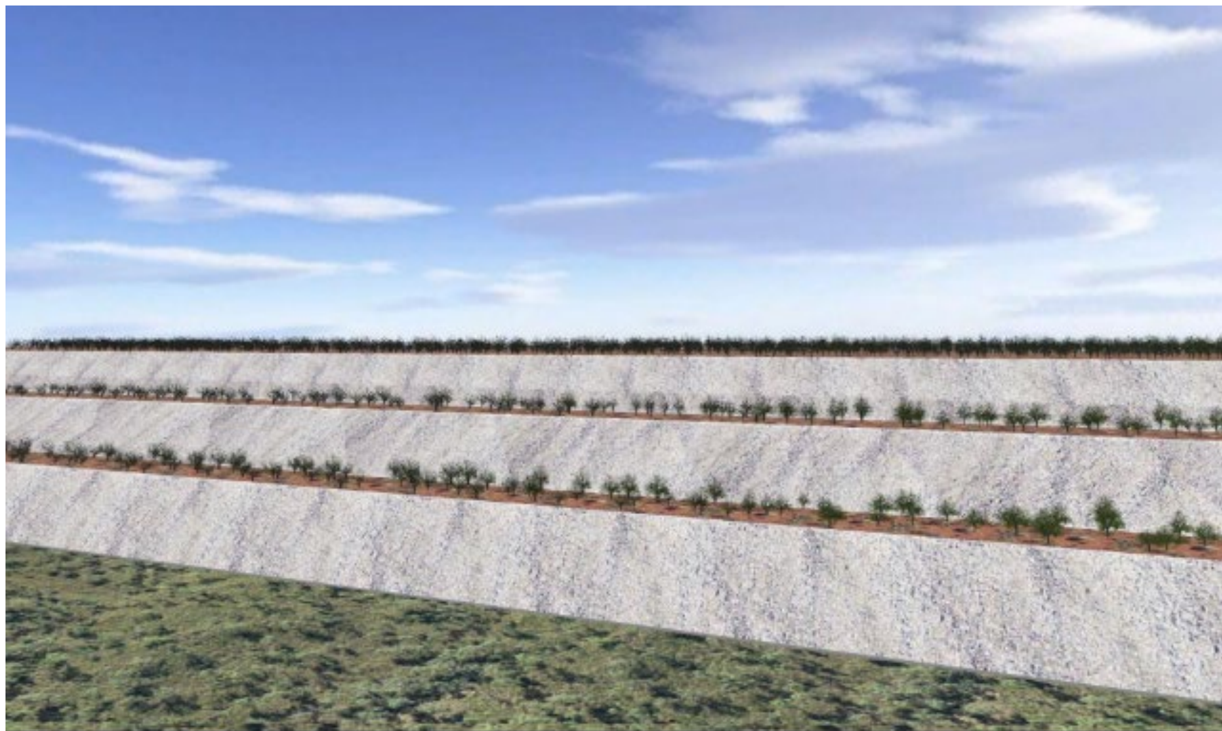
Figure 129 WRL batter design 2 - Battered and berm slope.
