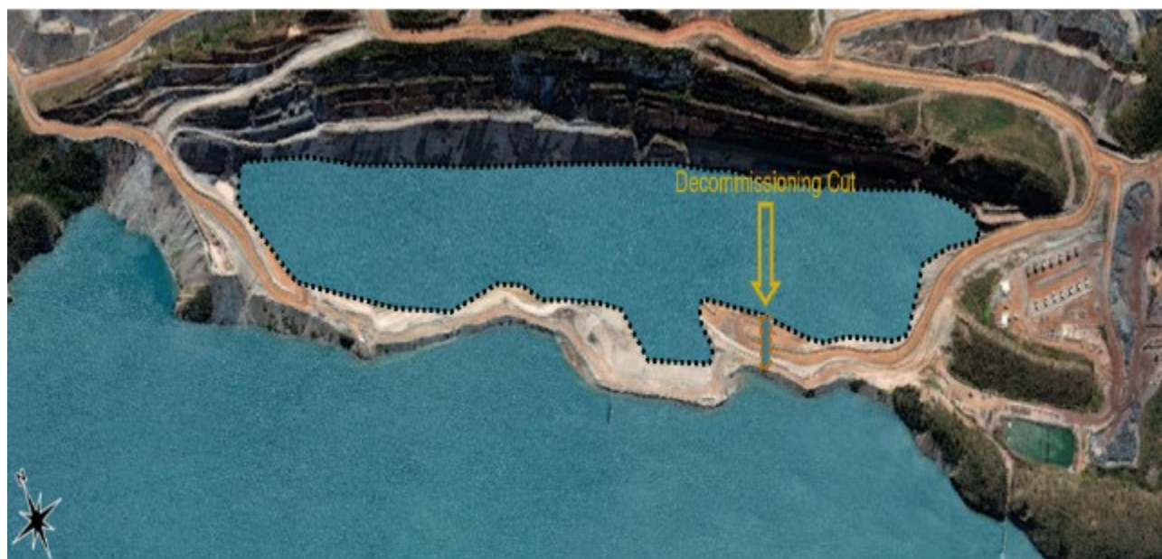
Figure 117: Conceptual location of the Decommissioning Cut (location, size and water levels are all approximated).
