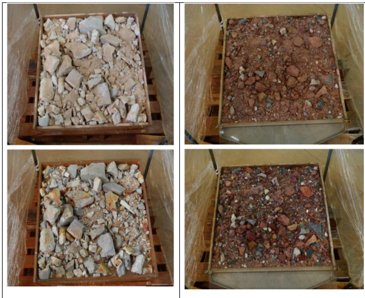
Figure 14 Quartzite (LHS) and WD1 Siltstone (RHS) before and after rainfall simulation
