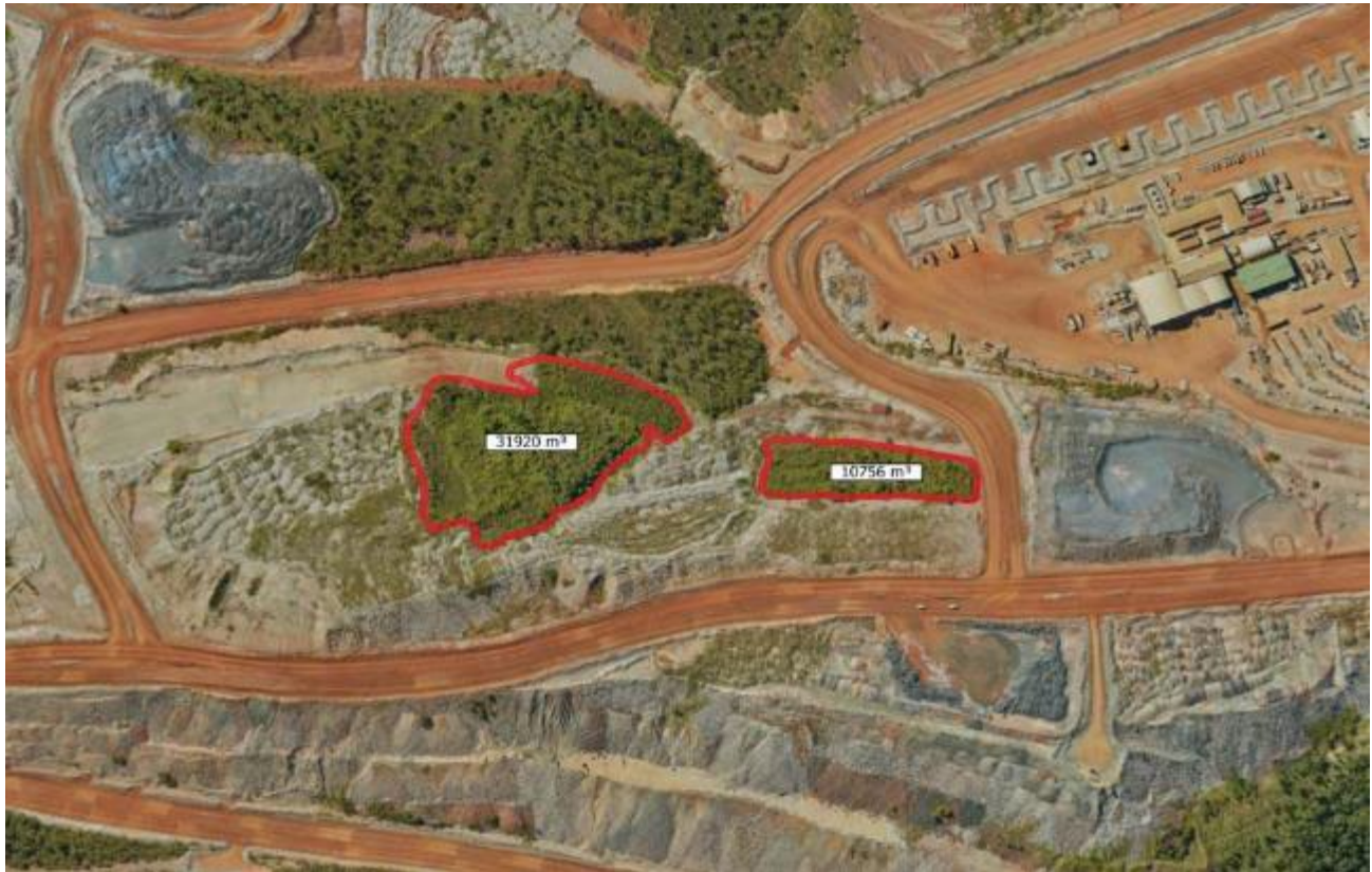
Figure 21: Location and Volumes of Topsoil Stockpiles on WD2
