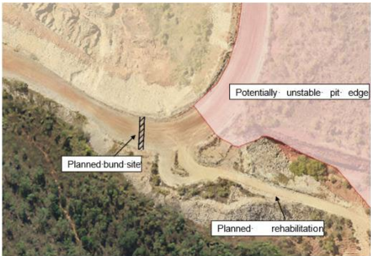
Figure 115: East Pit Abandonment Bund Location
