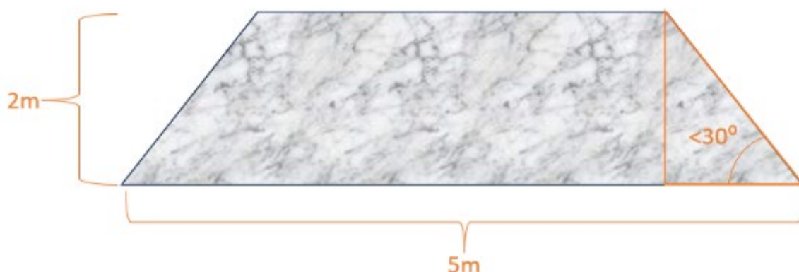
Figure 107: Minimum Specification of an abandonment bund
