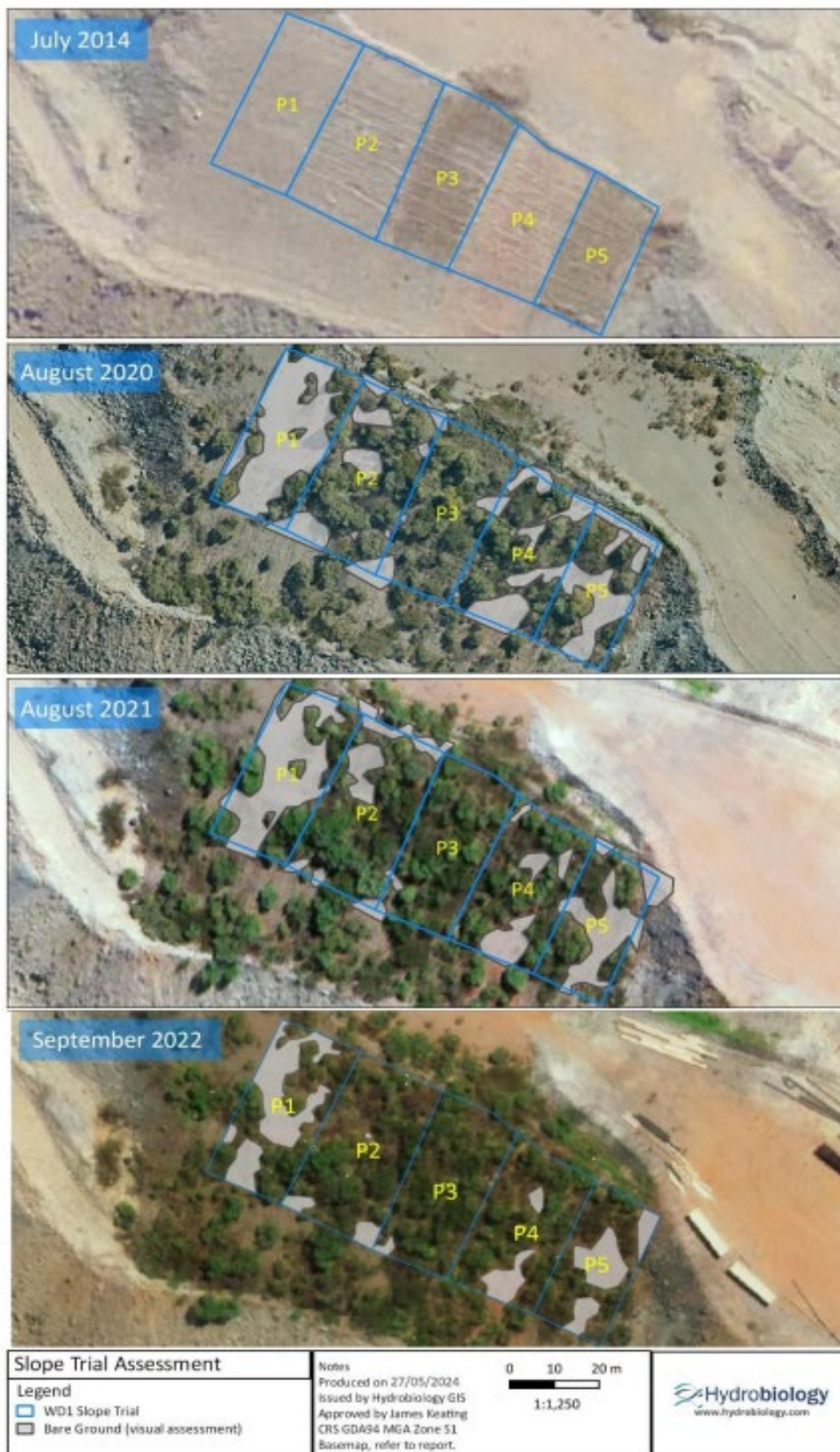
Figure 73 WD1 slope trial, with bare earth differentiated from vegetation cover by visual assessment.
