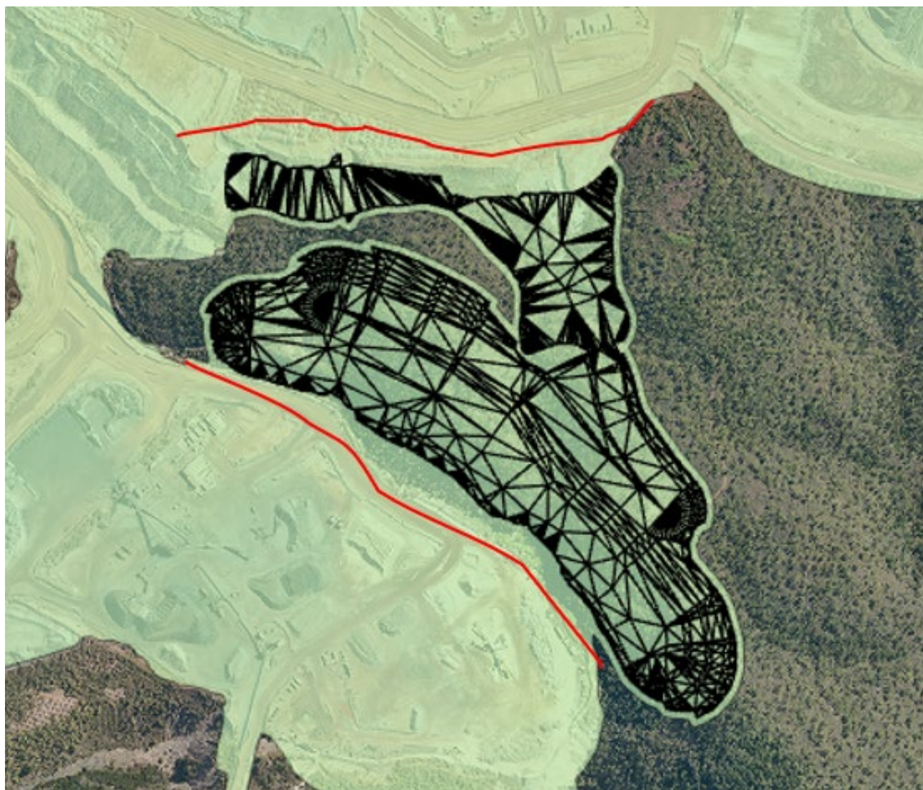
Figure 67 Conceptual location of the Mangrove deposit planned pit abandonment bund.
