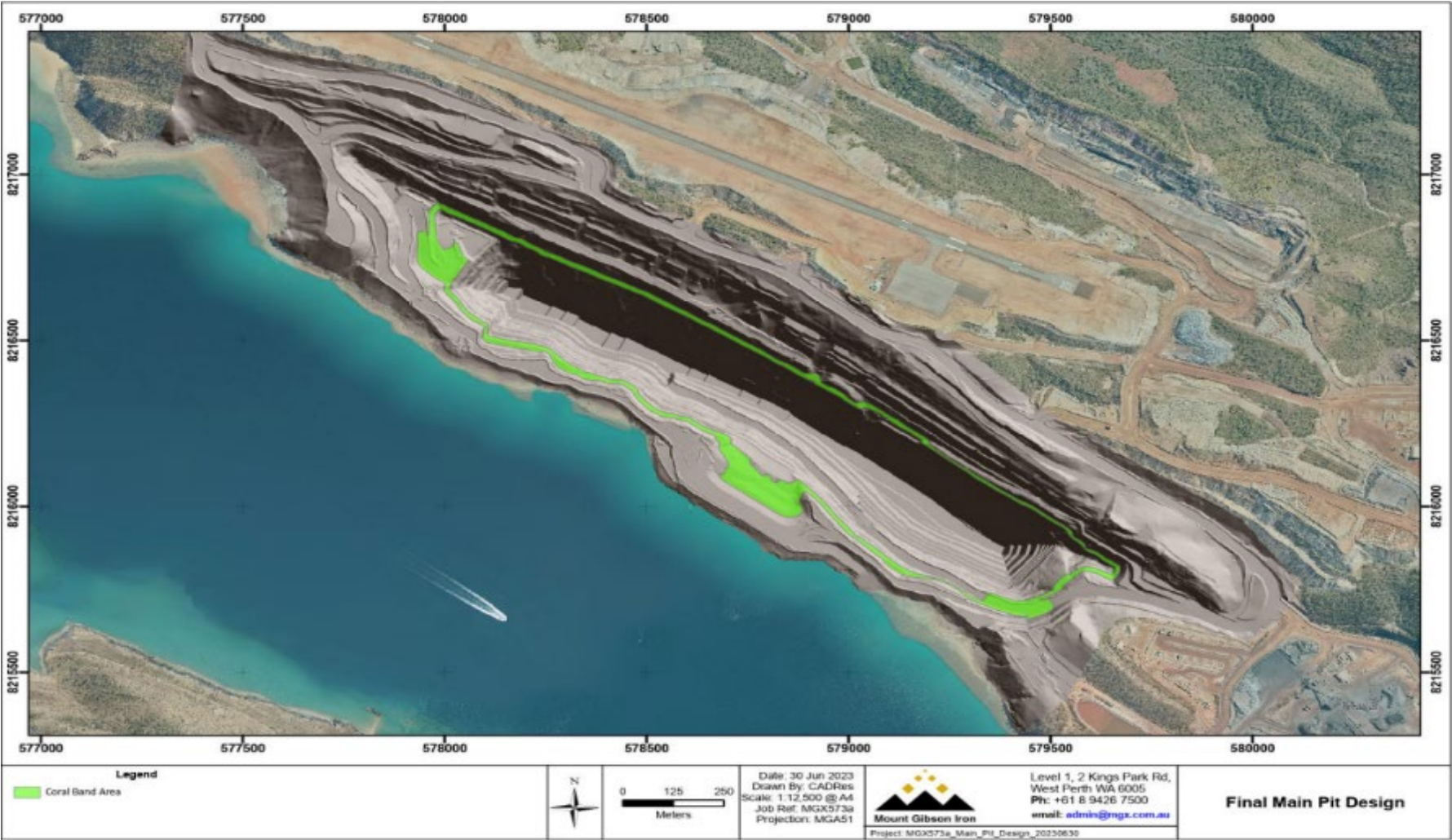
Figure 110 Conceptual closure over Main Pit. The green band represents benches potentially available for coral habitat as they occur in the forecast photic zone.
