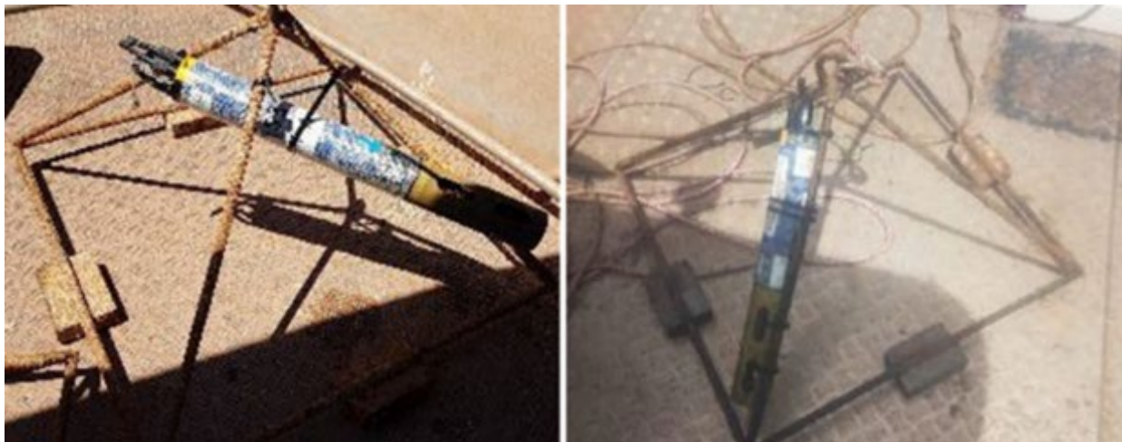
Figure 43: Remote submerged data logger (SDL) EX02 (left) and EX03 (right) water quality sondes, attached to custom weighted frames prior to deployment
