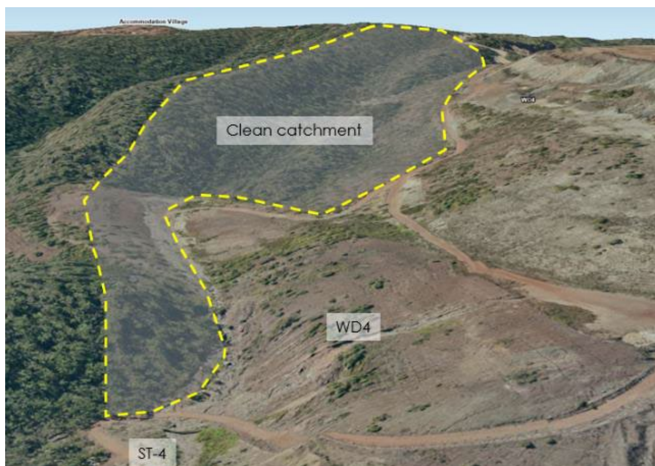
Figure 28: Clean sub-catchment on north side of Pindan Creek reporting to Sediment Trap 4
