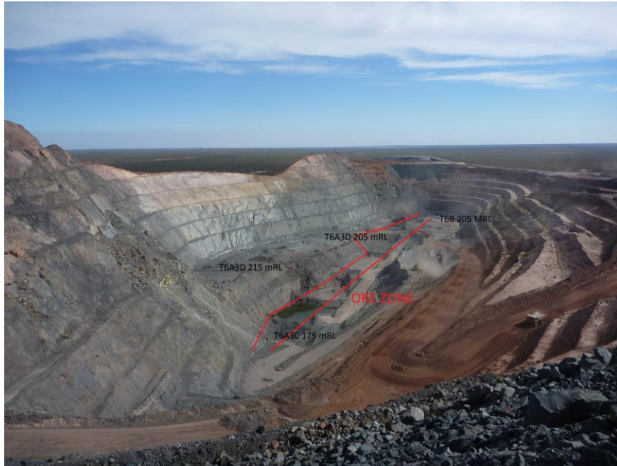
Figure 4 - Main Range pit at the end of March 2012. The ore zone is shown in red.
