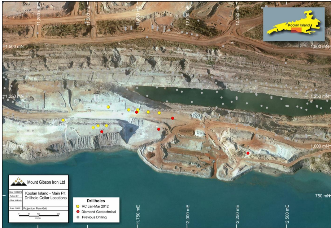
Figure 6 - Collar locations of previous and planned drilling in Main Pit. Collar locations of RC resource infill holes drilled in January to March 2012 are shown in yellow, diamond holes are shown in red.
