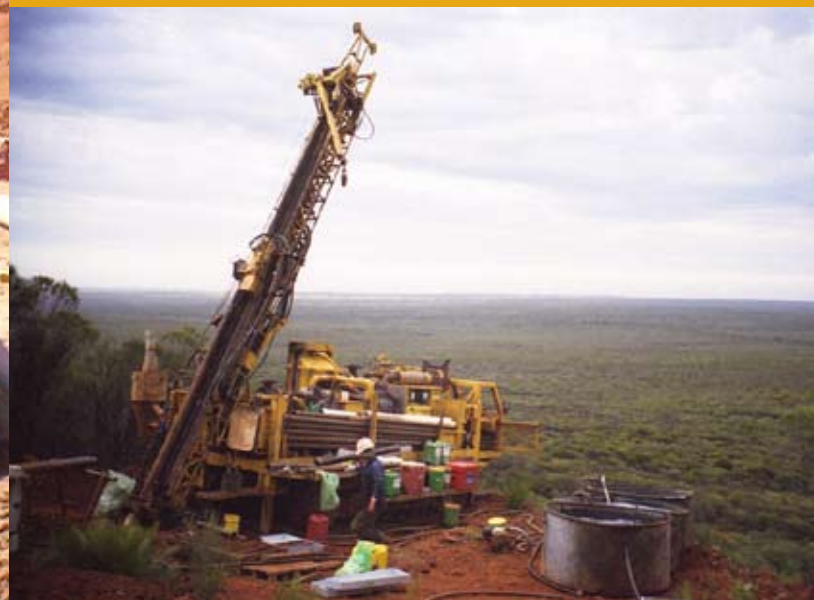
Figure 5 - PQ diamond core drilling at Extension Hill March 2006
